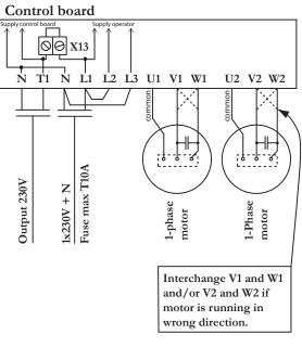
If a symmetrical single-phase motor is used (as shown on the left) make the following changes.
