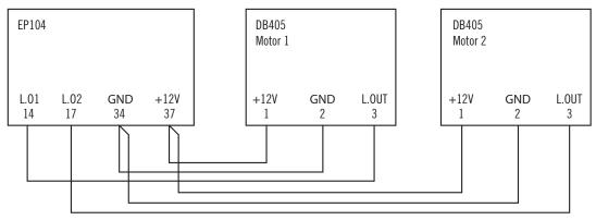
• Connecting a mechanical limit switch (microswitch)
