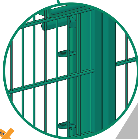
Padlockable drop bolt detail
