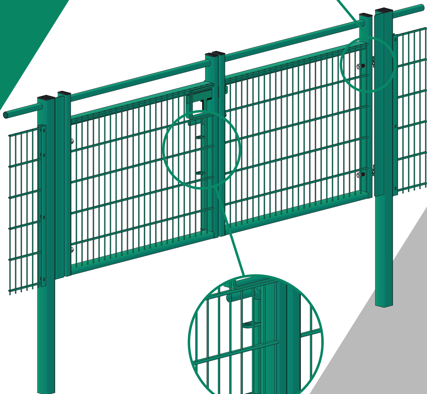
Padlockable drop bolt detail
